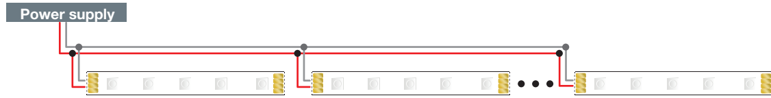
ELECTRICAL CONNECTION: connections in series or parallel
